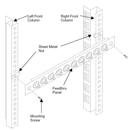
Refer to the illustration above. The BNC panel occupies 1 EIA unit (44 mm). The panel is designed to attach to the center hole within the EIA envelope.
